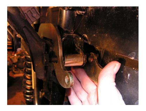
7.) Disconnect the sway bar from the frame. Placing the supplied drop bracket between the frame and the sway bar mount. Install the supplied bolts and repeat on other side. Tighten bolts after both sides have been installed.
